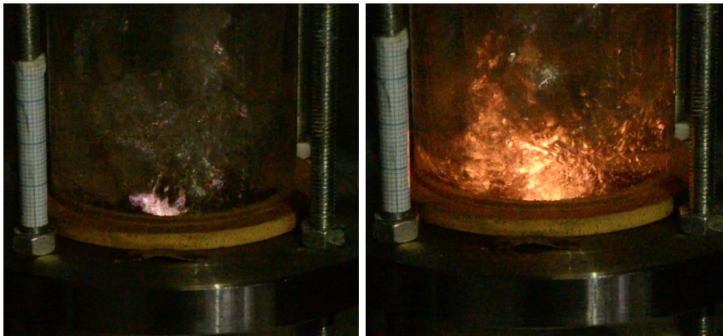
Rotating gliding discharge submerged in distillate. I = 160 \text{ mA} , Air = 20 L/m
